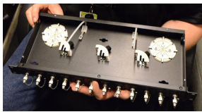
Custom 1RU fiber tray at STAPLES Center
