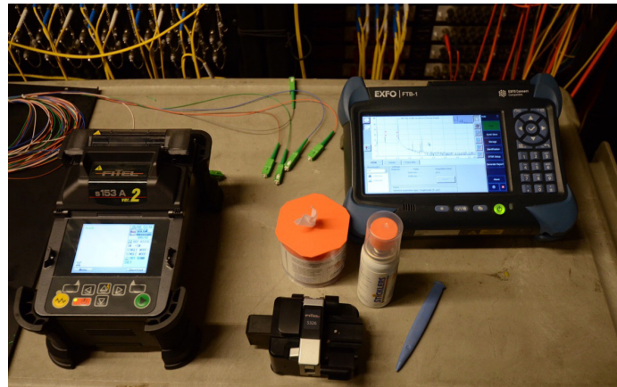
Examples of fiber-splicing equipment at STAPLES Center
